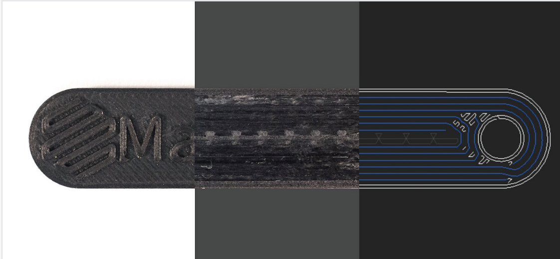
A cutaway view of our carbon fiber reinforced sample part and its layout in our software. The printer lays continuous strands of carbon fiber inside the part to provide increased strength and stiffness.
