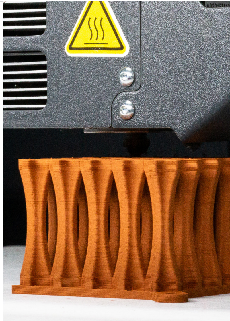
Heatsink 3D printed in pure Copper.
