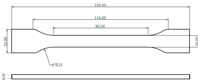
Tensile testing specimen; ASTM D638 (ISO 527, GB/T 1040)
